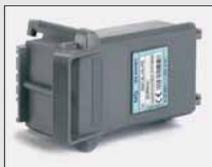
Tap-off box complete with terminals for cables of up to 25 mm<sup>2</sup>. Made from self-extinguishing plastic material, high mechanical resistance and resistance to static currents. The Box can be connected and disconnected when energized. Capacities from 16A to 32A.
