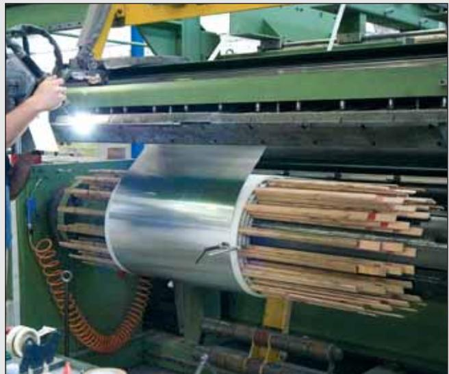
TIG welding in controlled atmosphere for LV connections.
