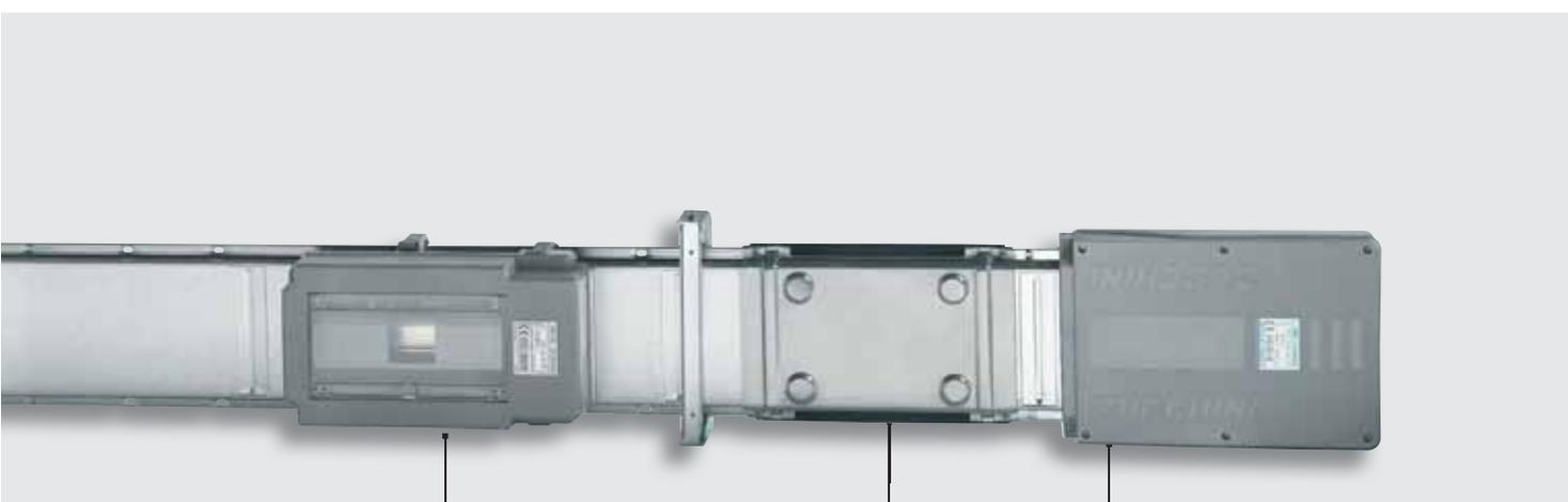
Tap-off box complete with terminals for cables of up to 25 mm<sup>2</sup>. Made from self-extinguishing plastic material, ensures high mechanical resistance and resistance to static currents. Plug-in type boxes can be inserted and removed when the busbar is energized.
