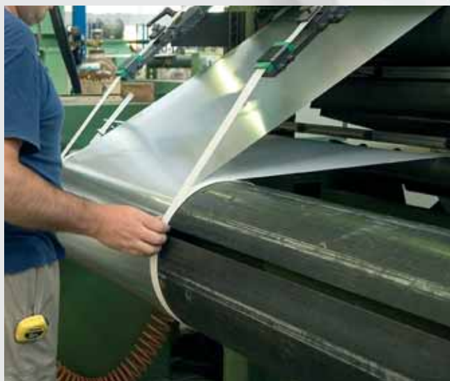
LV winding system
