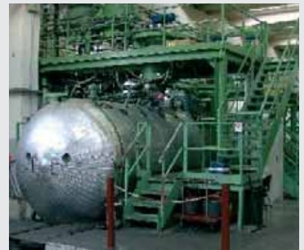
The pouring system under high vacuum.
