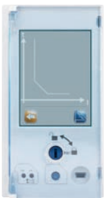
Earth fault tripping curve preview
